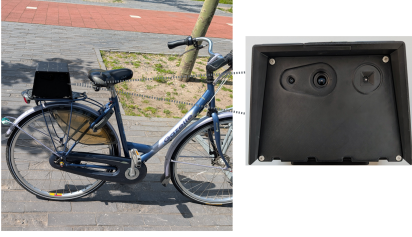
Fig. 1: The UrbanScape device with three imaging sensors and its deployment on a bicycle with magnets.
